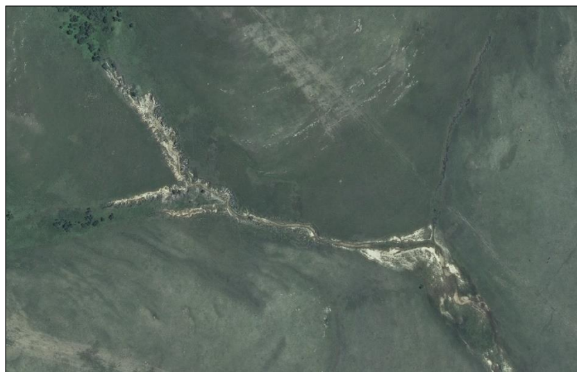
Figure 16. Example of an eroded upstream riverine wetland and downstream deposition
