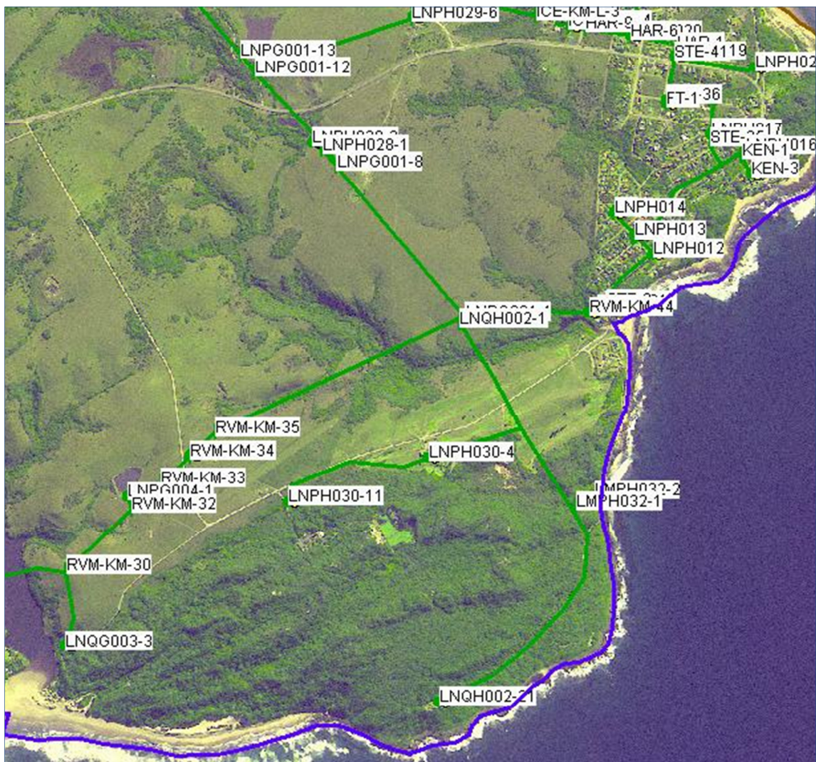
PLAN NO. 13: : Existing Sewer Reticulation
